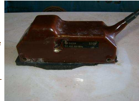
Figure 1: Damaged satellite transmitter showing bullet hole
